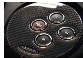
Carbon Shift Switch Panel
