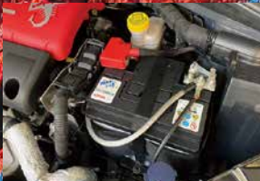
MTA Ground Cable
